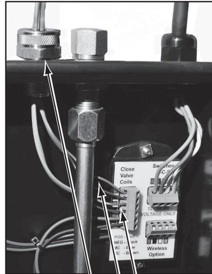
**3** [ ] Route the check valve cables through the connector parts. Then connect either cable to the top red and black marked connectors and the other cable to the remaining red and black connectors.
