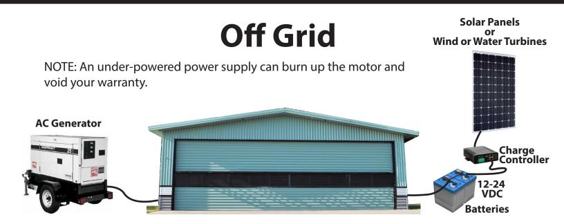
Electrical service is provided by you, using a gasoline, diesel, or natural gas driven generator to produce AC power. Some people use solar or wind or water power to produce DC electricity. This consists of solar panels or wind or water turbines, a charge controller, and batteries.
