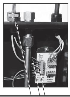
**3** [ ] Route the check valve cables through the connector parts. Then connect either cable to the top red and black marked connectors and the other cable to the remaining red and black connectors.
